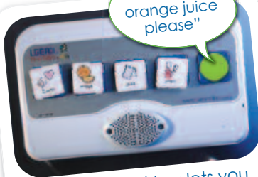
the speak all tag lets you say the sentence at the touch of one button
